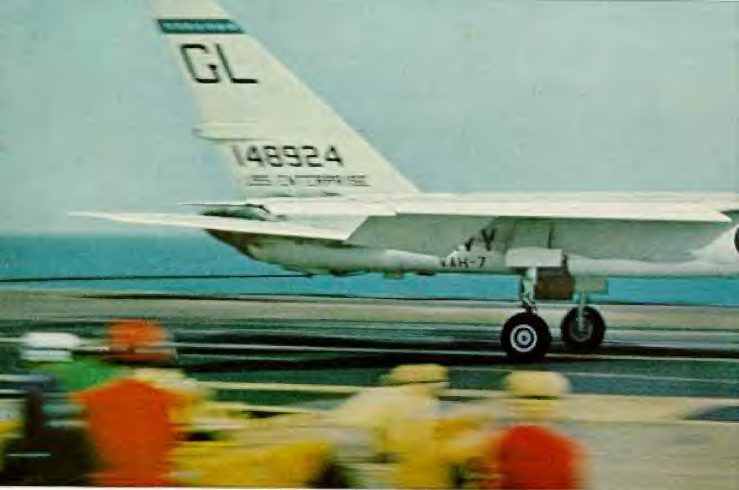
Twin jets howling, A-3A Vigilante (formerly the A3J) touches down on Enterprise's deck. An arresting cable snags on a hook under the tail and halts the plane.
