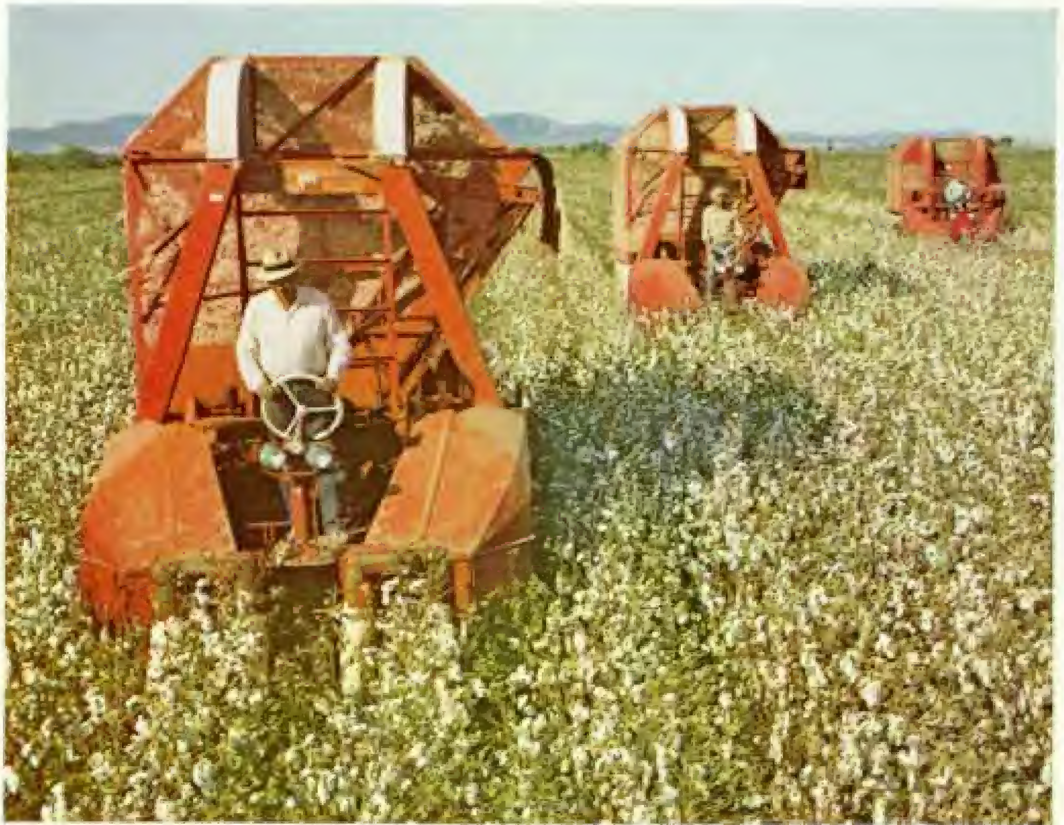
Combing a cotton field in Yuma County, a mechanical picker does the work of 110 men in a day. Cotton is king of Arizona crops.
