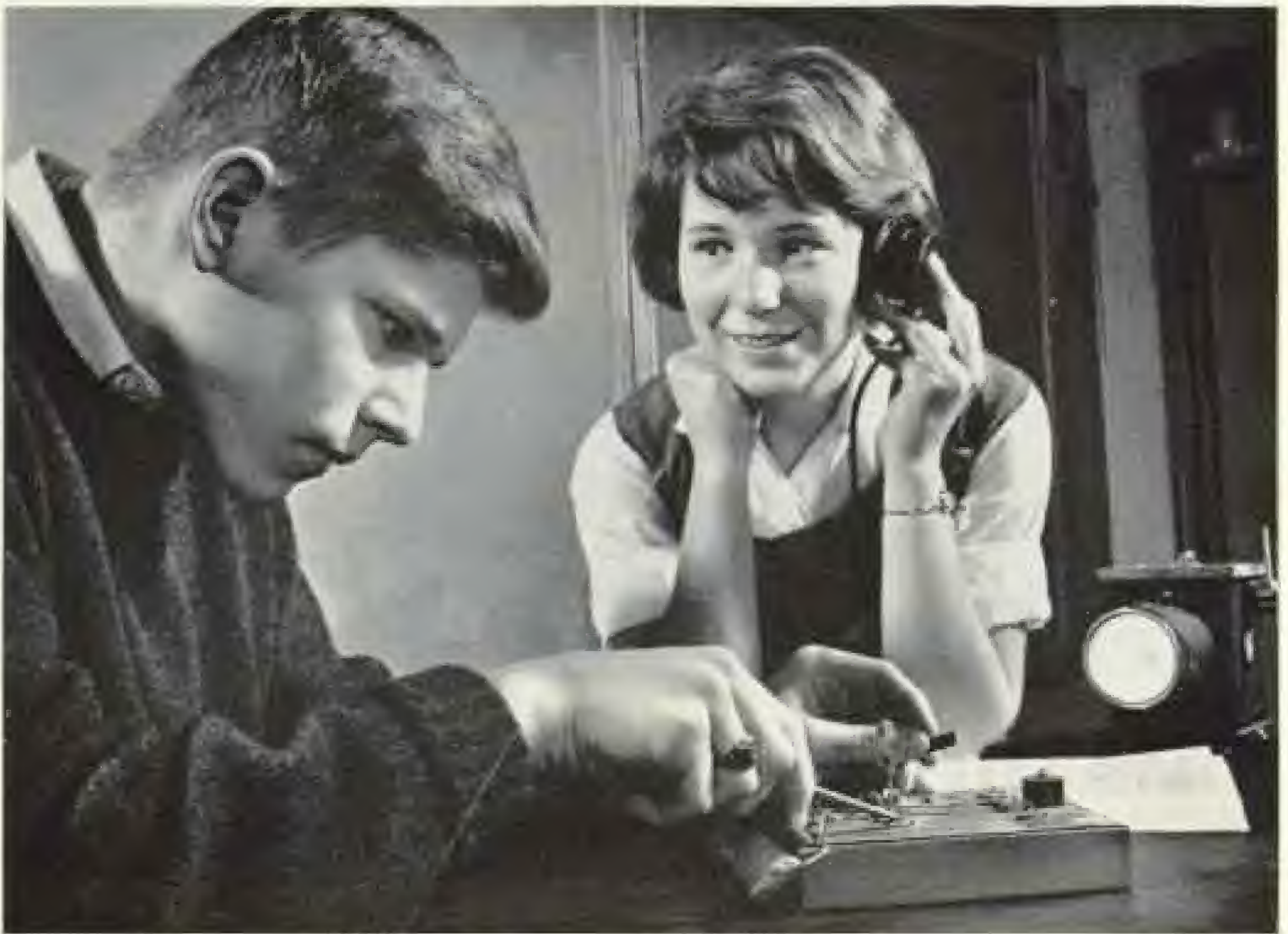
Two advanced physics students are producing a solar-powered, transistor audio-oscillator—the "From Sun to Sound" experiment—provided by the Bell System. The experiment requires students to calculate and design as well as construct some of the basic electronic components.
