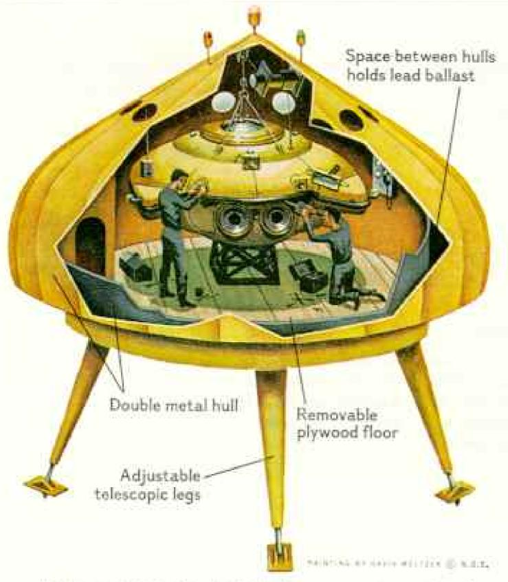
Like an oyster in its shell, the diving saucer hangs from the garage roof for servicing. Pedestal keeps her from swaying. Folding floor covers the open water through which she enters and emerges. Trials in the Red Sea amply proved the feasibility of hidden undersea pens for submarines.
