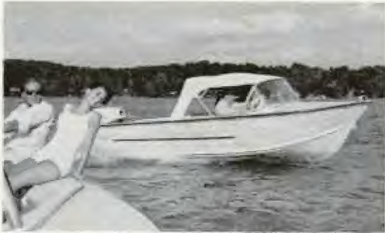
Jupiter-V 16 ft. concave-vee lapstrake aluminum hull.
