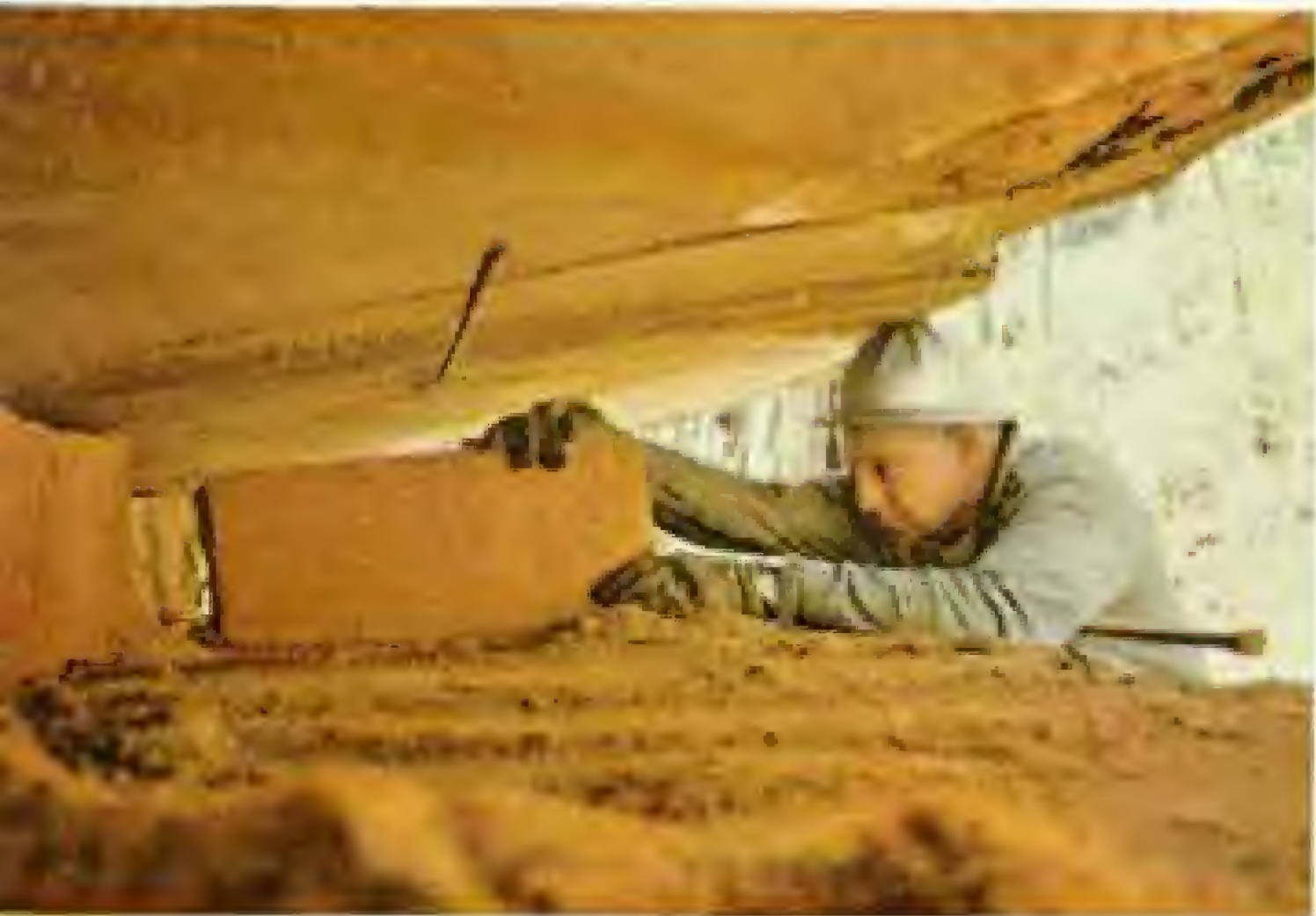
Screaming teeth of a chain saw sink into a coast redwood near Scotia. Steep slope forces the logger to make his cut high on the downhill side. Fellow worker (below) clears a cavernous notch that aims the brittle behemoth's fall toward a cushion of earth loosened by bulldozing.
