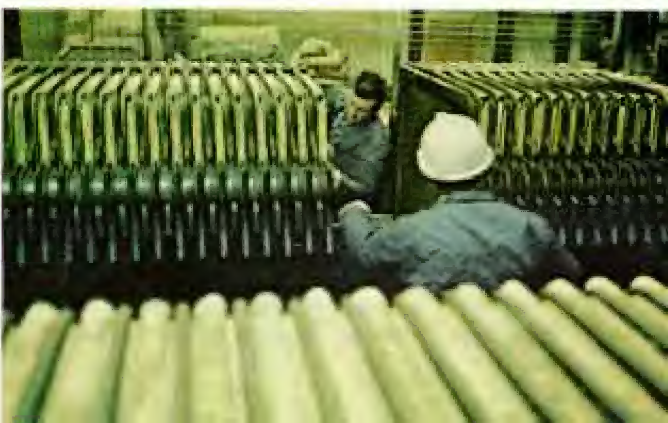
Clear solution (above), mixed with zinc dust, flows into filter presses (below). Zinc-gold compound emerges (above right).
