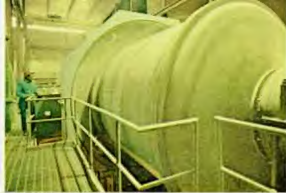
Rotating grinder reduces crushed ore to sand.
