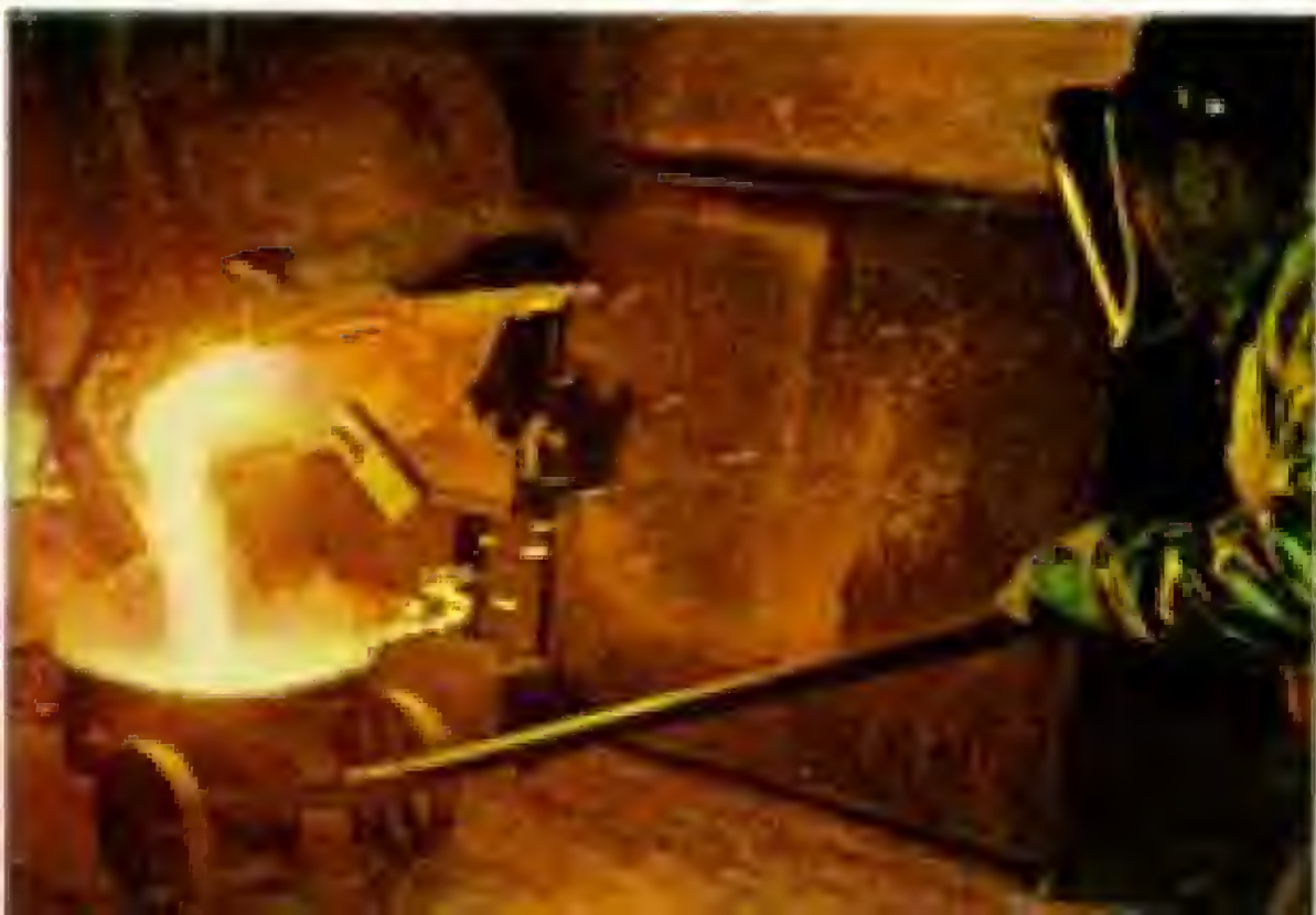
Glowing furnace smelts a gold "button," about 95 pounds.
