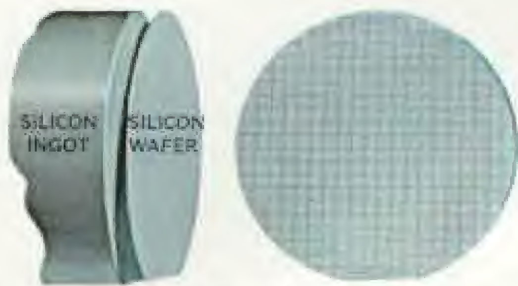
Slices of silicon ingot house the circuits
