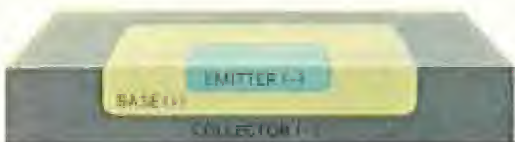
Furnace heat diffuses circuit elements into wafers
