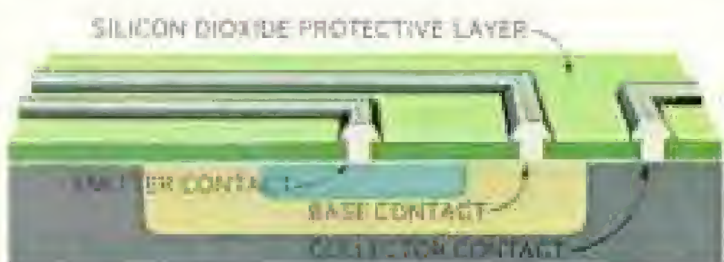
Simplified diagram shows a transistor in cross-section
