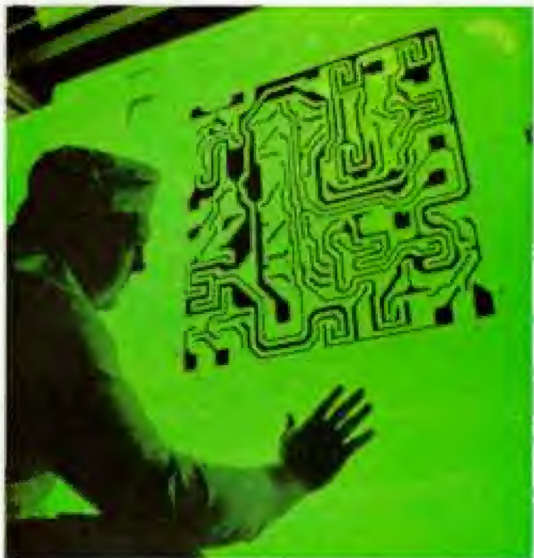
Plastic mask, when vastly reduced, will plot "wiring"
