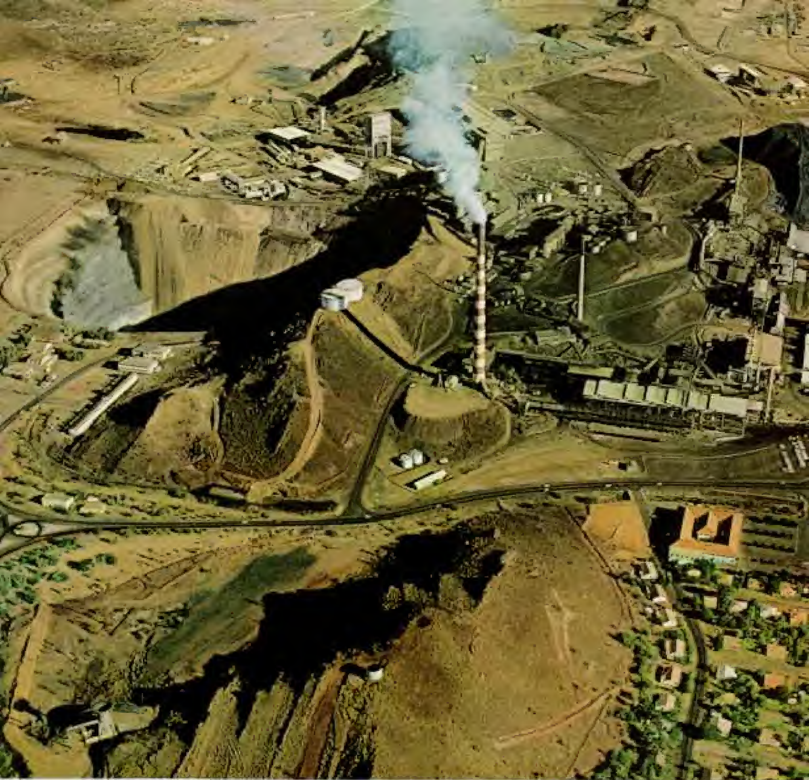
Industrial oasis in the outback, a vast mining complex at Mount Isa draws lead, zinc, silver, and copper from the red earth. Candy-stripe stack rises 503 feet above furnaces that smelt blister copper for refining in distant Townsville (right). Like blocks of Brisbane transplanted,
