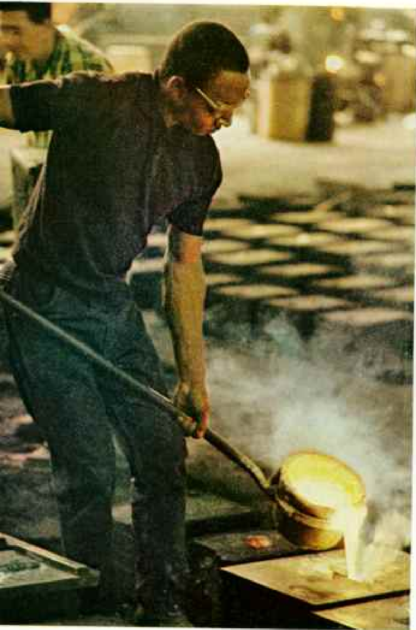
Spoon-feeding a mold with molten brass, a foundryman casts candlesticks at Virginia Metalcrafters in Waynesboro. Founded in 1890 to make stoves, the firm has kept craftsmanship alive with reproductions of 18th-century antiques.
