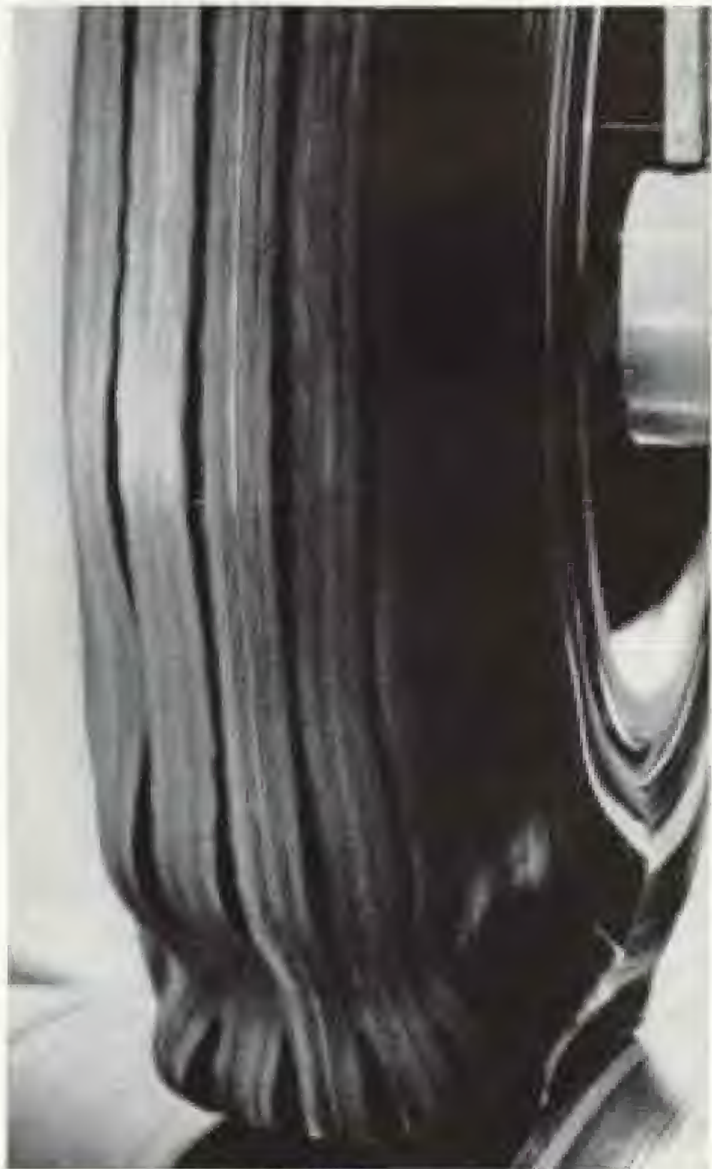
This is squirm at high speed. We run this conventional two-ply tire in our laboratories at exaggerated speeds (under rated conditions) so you can see how bad tread squirm can get. Notice how the tread surface of this two-ply tire is badly distorted.
