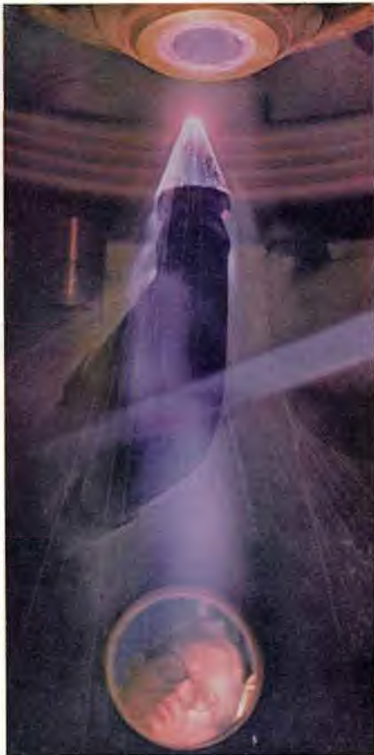
Gases heated as high as 10,000° F. pour over the model of a nose cone in a chamber at Sandia Laboratories in Albuquerque. From a porthole Nigel Hey observes the test, which helps researchers design space vehicles capable of withstanding heat generated by re-entry into the earth's atmosphere. Sandia Corporation, a subsidiary of Western Electric, operates the laboratories for the Atomic Energy Commission. With 6,500 workers, it is the state's largest private employer.
