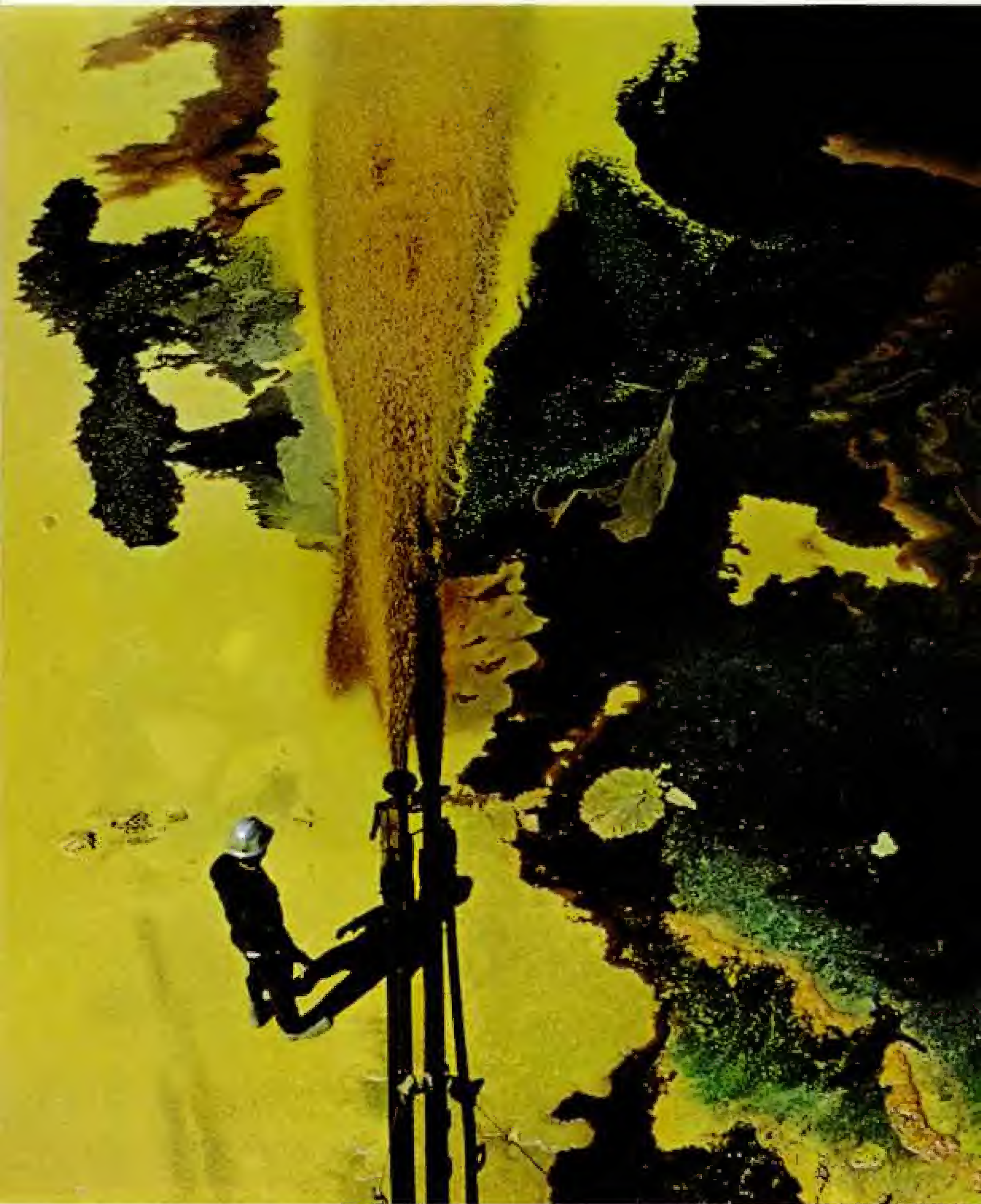
Golden gush of liquid sulphur spurts into a solidifying vat at Port Sulphur, where the Freeport Sulphur Company, world's largest producer, handles the output from five huge mines in the marshy delta area, two of them offshore. Powerful pumps force superheated water into the underground deposits; compressed air lifts the molten chemical to the surface.
