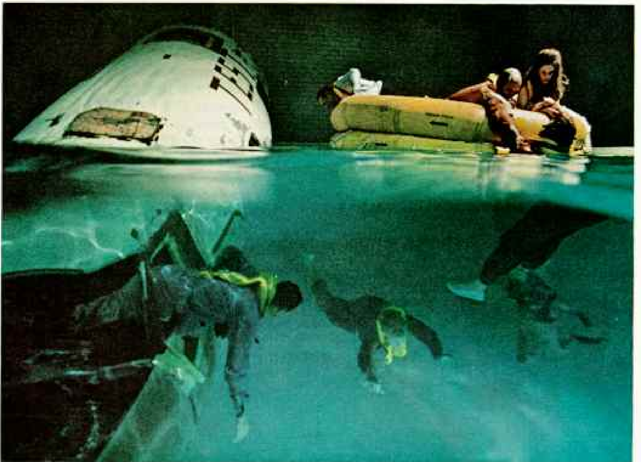
Seeking the best way to escape from a submerged plane, a test crew clambers out of an aircraft fuselage at the Federal Aviation Administration's Aeronautical Center in Oklahoma City. Dimly visible beneath the raft, a scuba-equipped lifeguard keeps watch. Enveloped in flame (right), FAA scientist Ernest B. McFadden tests his own invention—a plastic hood that protects the wearer from breathing flames and toxic fumes, allowing him time to get out of a burning plane.
