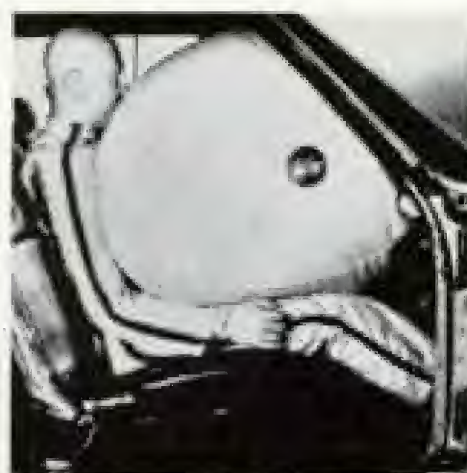
In a serious crash, air bags automatically inflate, save your life, and deflate—all in about half a second.
