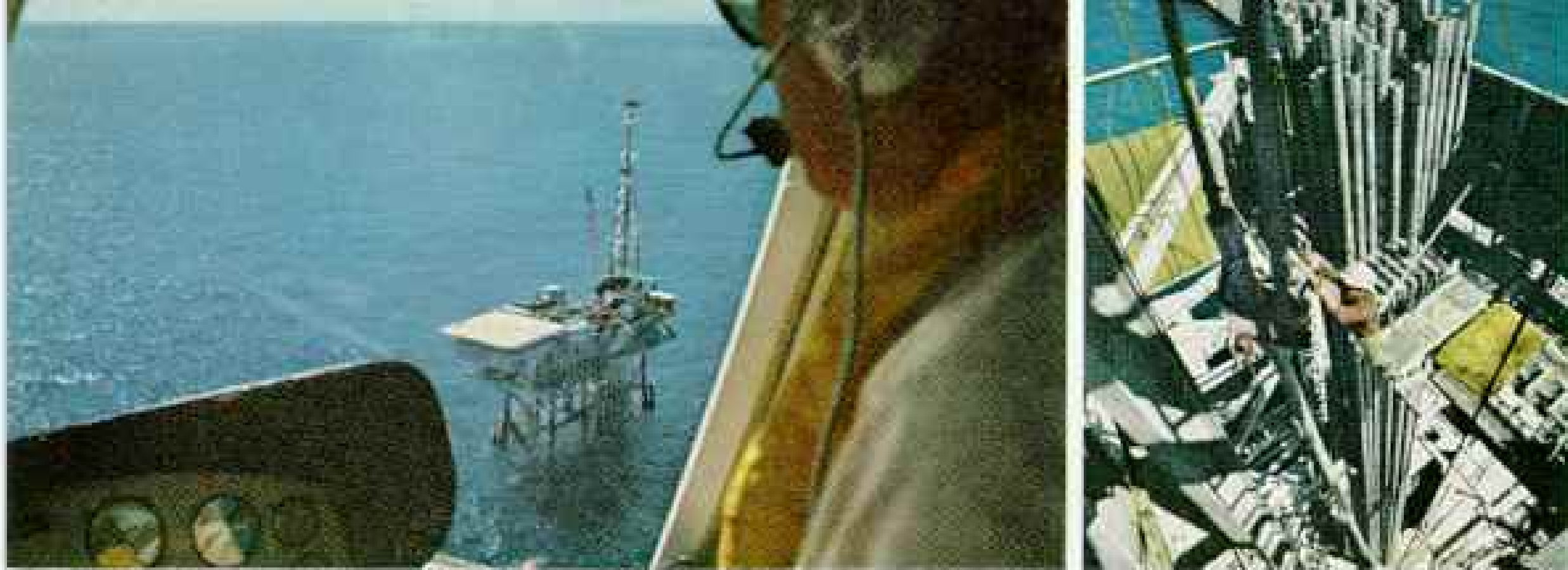
(Left) Helicopters carry small equipment and men to the rigs. (Right) To replace a worn bit, the entire drill pipe is taken apart, stacked in the derrick, and then reassembled. Drillers call this "making a roundtrip."
