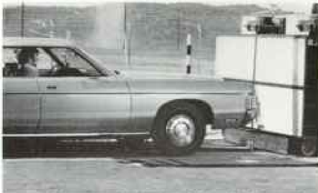
Car approaches barrier at 17-mph. (Man wearing lap belt only.)
