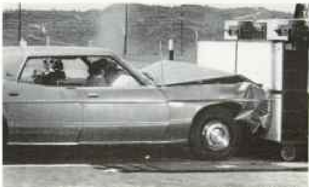
Air bag cushions man, prevents injury 4/100ths of a second after impact.
