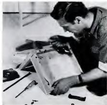
STEEL CORNER BRACKETS give furniture strength, are bolted on. The swivel chair is assembled in 15 minutes.
