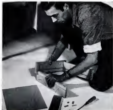
PRECUT GROOVES permit parts of the drawer to slip together. All of the pieces are joined in the same way.
