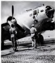
near point of detonation. Long cable with floats (center) collected water samples. At right, radioactive dust is washed off a B-17 which flew through atomic cloud.
