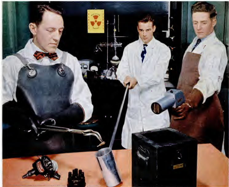
In this "Radioactive Materials Room" at Chrysler Laboratories, many stronger metals . . . better designs . . . smoother-running, longer-lasting parts have their beginning. Note the protective lead-and-rubber gloves and aprons, and the thick lead box in the foreground where "hot" parts are safely stored.
