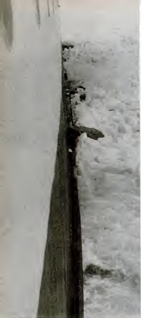
ICE AND SHIP got along well together. Sides were scraped but vessel suffered no structural damage.
