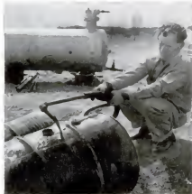
POURING OIL from his main tank (background), Welch lifts the nozzle as the drum fills. Drum holds 55 gallons. A barrel, the standard measure, holds 42.
