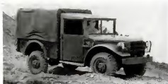
This M-37 cargo carrier, built by Chrysler Corporation, can travel more rapidly and surely over rough country than our World War II cargo carriers. The ride is steadied for men and cargo by new suspension principles, improved springs and heavy-duty shock absorbers that provide extra cushioning power on bad roads or roadless terrain.
