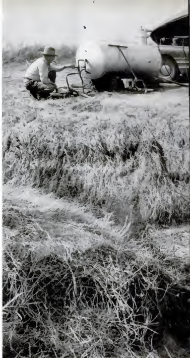
WELCH'S PUMPING RIG is spectacularly simple. Here Welch (foreground) tightens connecting hose on Well No. 2, a four-foot hole in which he has sunk a perforated two-inch pipe. Oil is sucked through pipe and hose into the vacuum
