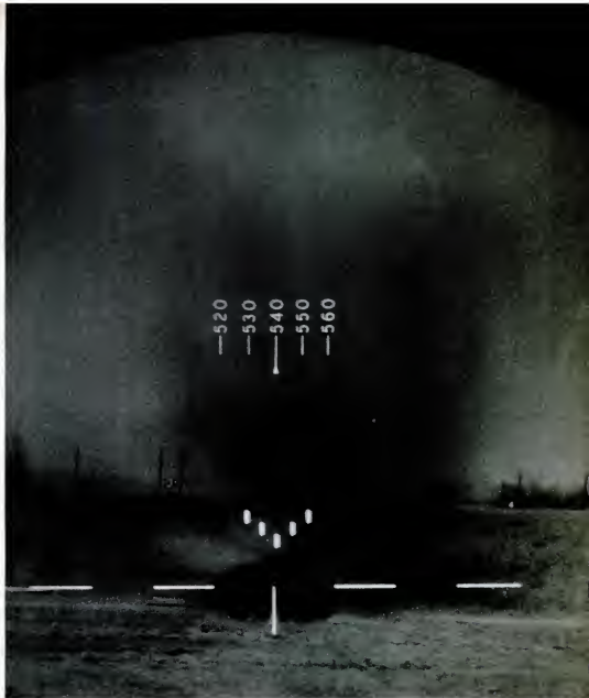
THROUGH THE SIGHT , the M-47's gunner aims the 90-mm gun by placing top of heavy vertical line
