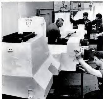
GASOLINE TANKS are made in odd shapes to fit around the M-47's engines. Two tanks (center and left) then go into each chassis, hold more than 250 gallons.
