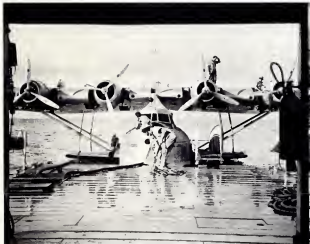
9 Servicing the Clipper at Midway. At each island the ship is inspected at night and prepared for the following day's flight. Parts of the wings open up to give footing to the crew of mechanics checking the 800-h.p. engines.
