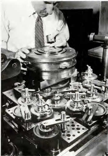
Geometric lathe makes fine patterns and scrolls. A diamond cutting point remains stationary while gears move bed forward and backward. Gears simultaneously move pattern-making wheel.
