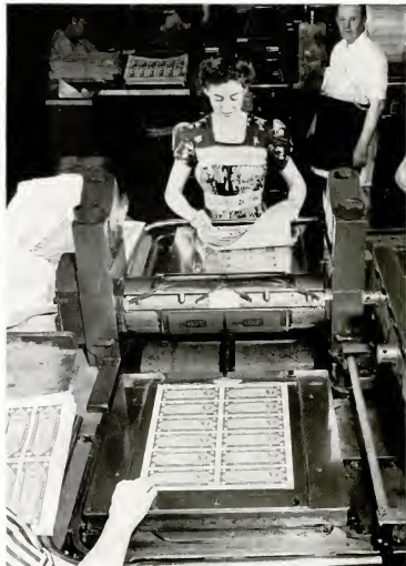
Flat-bed press prints notes. Plate goes through inked rolls, then after moving through roll of absorbent paper it is wiped by hand, removing excess ink, and finally prints sheet of twelve notes.
