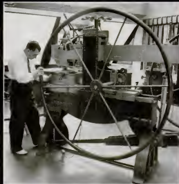
Transfer press is used to transfer the engraver's portrait to the master plate. The portrait is assembled on the steel master die and
