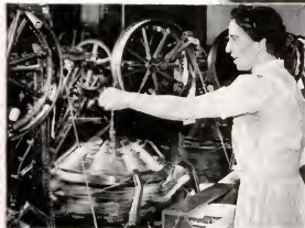
Her Son Was At Pearl Harbor , so patriotic Marie Meyer is now devoting her energies to war production at a General Electric factory. She operates a machine braiding colored covers for aircraft wiring. Mrs. Meyer says, "Making things that help our boys win the war is a great comfort to me."
