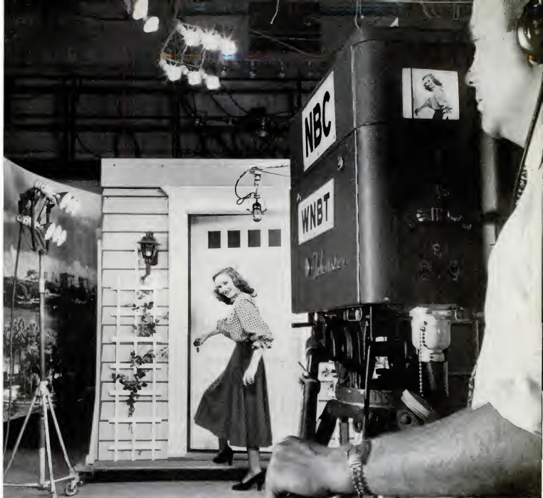
TELEVISION-CAMERA VIEW FINDER (UPPER RIGHT) SHOWS HOW AUDIENCE SEES ACTRESS EVA MARIE SAINT. MICROPHONE AND LIGHTS ARE CUT OUT AND THE CHEAP SET LOOKS REAL
