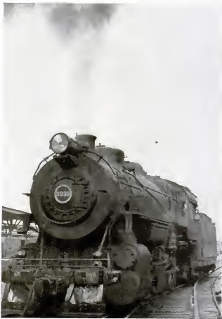
SAME LOCOMOTIVE emits almost no smoke when special steam jets, installed in firebox, force air into smoke-forming gases and burn them away.
