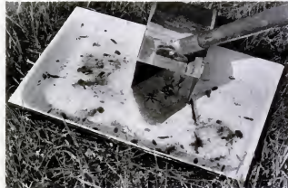
BUG COLLECTING is done with a Tarnwell surface sampler, named after the head of the project, which skims insects and larvae from stream's surface.
