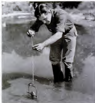
MUD COLLECTING is done with the ooze sampler. A small weight slides down string to release the compressed bulb of a syringe imbedded in the mud.
