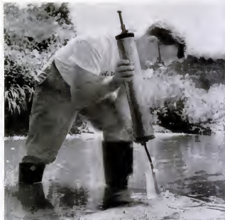
WATER COLLECTING is done with a big brass cylinder which holds two quarts of liquid. The water is then analyzed for its average oxygen content.
