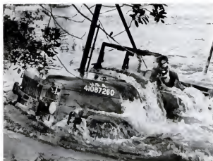
EMERGING from river, amphibian sheds water from its sealed engine. On land it can operate in temperatures of 65° below zero to 125° above.
