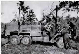
TRUCK'S BREATHING DEVICE consists of two pipes which protrude above surface, "snorkel" (right) for air intake to engine, "shorter" for exhaust.
