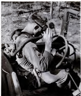
DRIVER'S BREATHING DEVICE , with compressed air tanks and mask, was developed by a French diver, Jacques-Yves Cousteau (LIFE, Nov. 27).
