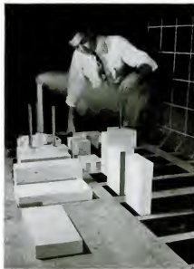
SMOG TUNNEL in New York is used to study the path of Consolidated Edison smoke as it blows past U.N. buildings which are being built near the plant.
