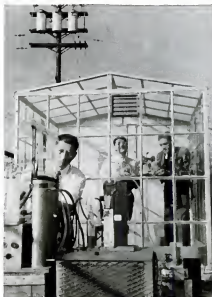
SMOG CHAMBER in Los Angeles produces smog (foreground) so scientists can test its effects on humans and plants and learn how much sun it cuts out.
