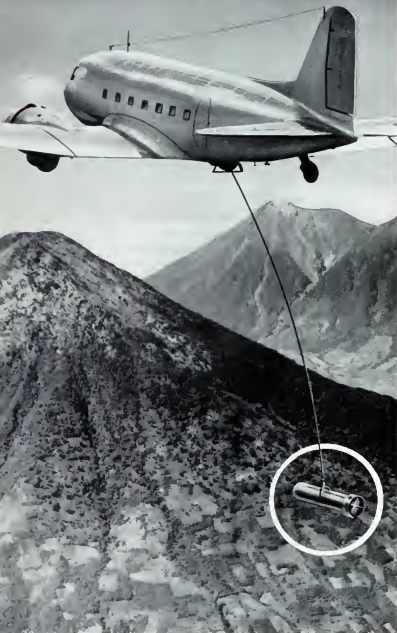
TRAILING BELOW THE OIL EXPLORER'S PLANE , the airborne magnetometer records the earth's magnetic field. Other new tests and devices are developed by thousands of oil companies in the race to meet oil needs. The driving force—competition; the result—a stronger America—more and better oil products for you.
