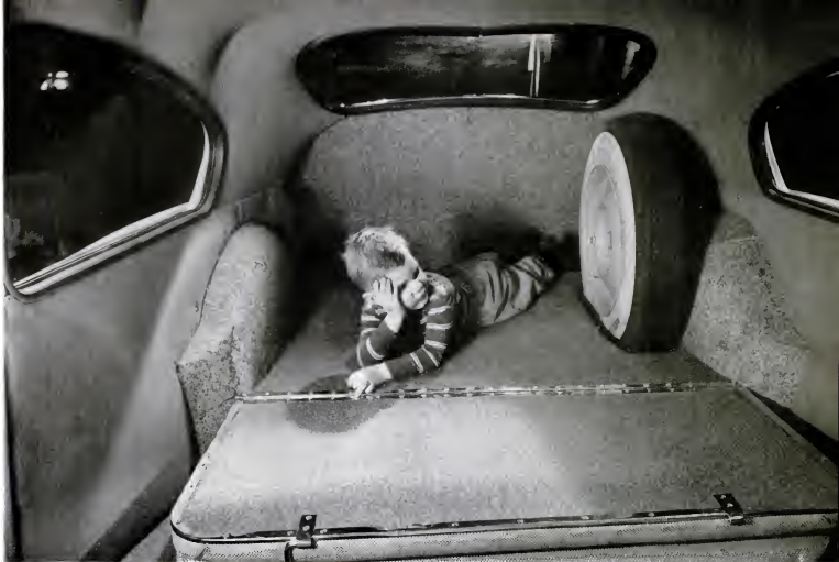
RED CAR'S BACK SEAT FOLDS FORWARD TO MAKE DOUBLE BAGGAGE SPACE. WITH THE SEAT UP, THERE IS STILL A 20-CUBIC-FOOT AREA WHERE BOY IS LYING
