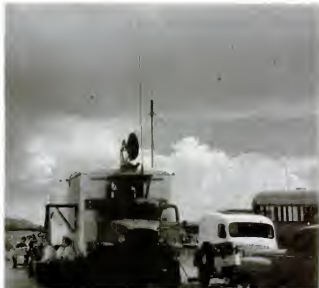
RADAR DETECTORS , focused on New Mexico cloud from mobile equipment, indicated by "echoes" that precipitation was forming within the cloud.
