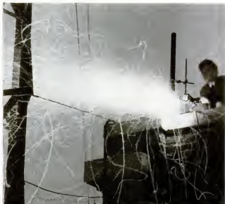
CHARCOAL BURNER was first used to vaporize silver iodide in method invented by Dr. Bernard Vonnegut (right). Later he perfected hydrogen torch.
