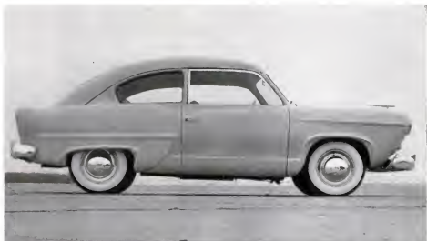
THE "RED CAR" is 60 inches high, has 100-inch wheelbase, standard tread width and extra-wide doors for easy
