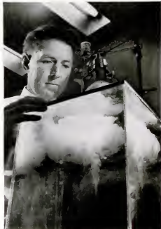
GLASS-WALLED CLOUD BOX , examined by Dr. Schaefer, is used to simulate natural cloud conditions.
