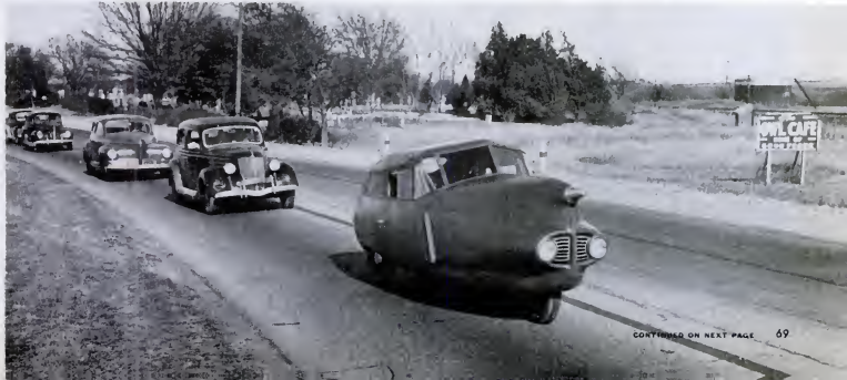
ON THE GROUND, WITH FLYING SURFACES OFF, ROADABLE PLANE IS A STREAMLINED, THREE-WHEEL COUPE, HAS A FOUR-GEAR SHIFT, DRIVES MORE THAN 60 MPH
