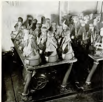
VIOLENT SHAKING of flasks on tables which move back and forth and around aerates the solution and helps organisms to grow. Shaking continues for three days.
