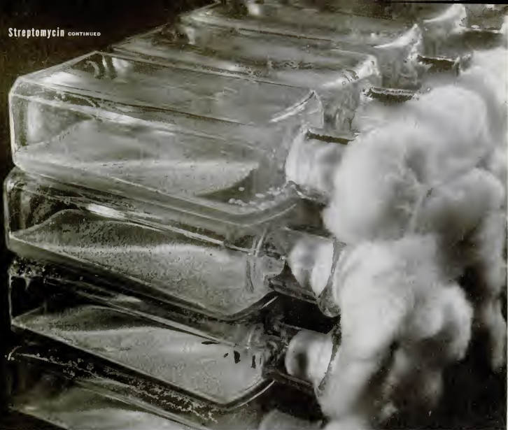
STREPTOMYCIN PRODUCTION starts with the introduction of a pinhead quantity of the streptomycin organisms into small bottles containing nutrient. Four-days'
