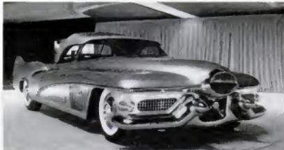
LE SABRE, experimental GM model built in 1950, was a test bed for new ideas. It was first to show wrap-around windshields now going into '54 Buick.
