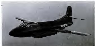
NAVY'S ALL-WEATHER JET , Douglas F3D Skyknight, mounts four 20-mm cannon. By the end of this year the Navy hopes to have it operating off carriers.
