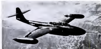
BIGGEST INTERCEPTOR , Northrop F-99, went into production last summer. It carries more rockets than other interceptors, can fly long-range patrol.
