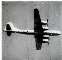
RUSSIAN BOMBER, TU-4 , was copied from B-29s which made forced landings in Russia during last war, were held by Reds. Propeller-driven, it has a range of about 4,500 miles carrying 5 tons of bombs.
