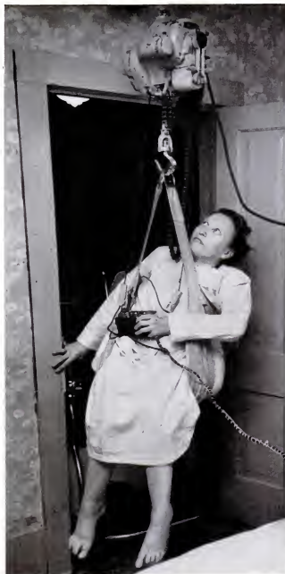
BEDROOM HOIST , which runs on overhead track, was built by twins' brother. It lifts Anna out of chair into bed. She operates controls herself.
