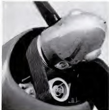
RUBBER BELTS, looking like auto fan belts, gear engine down to permit the propeller to turn at low speed.
