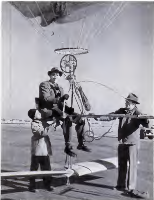
SOFT LANDING is effected when Paul stops pedaling. Machine will rise 300 feet, travel 14 mph. Direction is controlled by working the rotors, again as in a helicopter. One hitch: against a 14-mph wind, it makes no headway at all.
