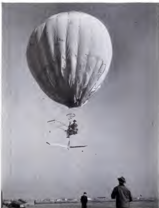
BICYCLE AND BALLOON combine to form Charles Paul's Pedalcopter in test at Lakehurst, N.J. Balloon reduces the weight of machine and pilot to 20 pounds. By pedaling, Paul works rotors to lift the contrivance like a helicopter.
