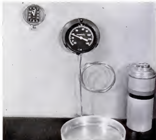
Temperature goes down as refrigerant begins to evaporate and disappear into air. Same principle is employed by body when perspiration evaporates from the skin.
