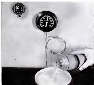
Evaporation is basic principle of refrigeration. Here Freon 12, a rapidly evaporating liquid, is poured into pan connected to thermometer which reads 79° at the start.
