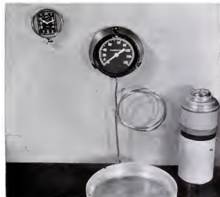
Pan is frosted and temperature is -14° after 80 minutes of evaporation. Because most refrigerants evaporate at room temperature they must be kept under pressure.
