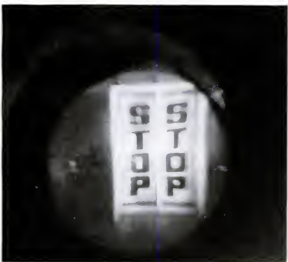
IN FOG TEST Fog-O-Scope is placed in front of twin STOP panels (top picture). Sky-writing smoke, simulating fog, pours from generator, obliterates sign at the right from vision (middle). But view of the instrument's screen (bottom) shows it has detected the hidden sign as well as the unfogged panel.
