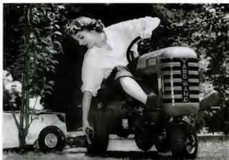
MANEUVERING around a small tree with Yard Hand is easy. Clutch in either rear wheel can be disengaged (above) so that the tractor turns in short space.
