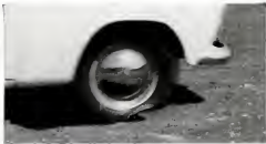
3. Ugh! It slams right into the sharp edge of the hole so hard the tire is crushed back to the rim.
