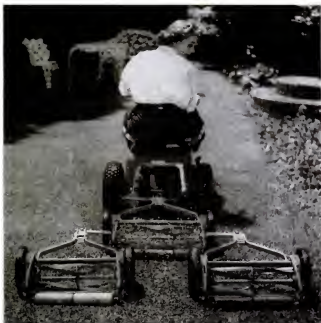
GANG MOWER consists of three mowers (one 18 inches, two 16 inches), will cut 45-inch swath of grass. It costs under $100, will be ready in September.
