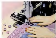
9. Basic set of attachments, including ruffler, binder, hemmer and gatherer comes with machine at no extra cost. Many others, including buttonholer shown above, available at small cost.
