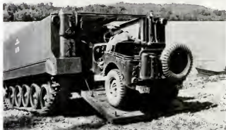
TAKING ON JEEP through rear door, M-59 prepares to go into the river. To increase floating ability, much of inside of 20-ton M-59 is lightweight aluminum.
