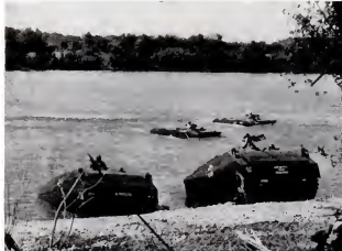
CROSSING RIVER , Lifesavers use land tracks to propel and steer since they lack both propeller and rudder. They have speed of only 4 knots at best.
