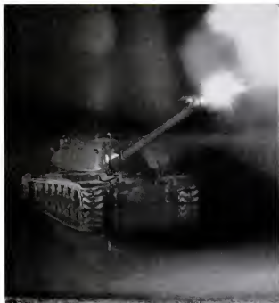
IN NIGHT FIRING EXERCISE big 120-mm gun of the T-43 cuts loose at Newark, Del. Tank's .30-caliber machine guns can be fired with main gun.
