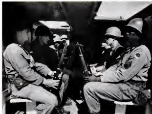
SITTING INSIDE LIFESAVER , an infantry rifle squad occupies benches which can fold to make room for bulk cargo. Two escape hatches are open.
