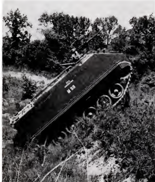
OVERCOMING ROUGH TERRAIN , M-59 climbs hillside. Principles of weight distribution which make M-59 float also make it ride with less shock.
