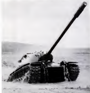
EASY TO MANEUVER , T-43 wallows in a crater, preparing to fire from it. With power steering, tank can be handled almost as easily as a farm tractor.
