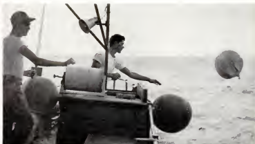
EXPLORATION CREW drops balloon buoys marking location of "geophones." Underwater charges are set off and geophones record sound waves to chart earth formations beneath ocean floor—pinpointing likely drilling sites. Just for the right to search, oil companies have already invested over 100 million dollars in offshore leases. Yet they still face years of work and millions in additional expenditures before they can hope to break even on offshore ventures.
