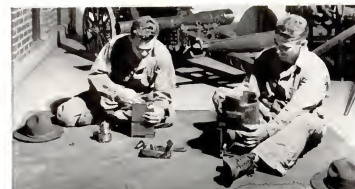
Breech parts of 75-mm. howitzer are cleaned by Lackey and Duckett. Gun weighs 1,270 lb., compared to field howitzer's 2,090 lb. With a 9,500-yd. range, it can throw six 14-lb. shells a minute.
