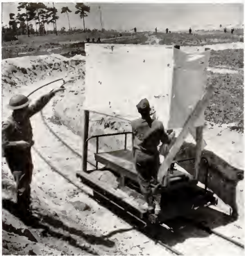
After firing, the railroad target looks like this. Powered by a gasoline motor, it runs along a winding, lumpy track. Recently three generals, out for a joyride, were tossed off on a curve.
