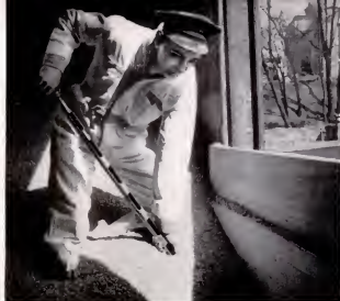
2 "This hollow pole-like device . . . 6 feet long, called a 'grain thief' . . . scoops out samples from top to bottom to insure that each grain shipment meets the rigid standards of Old Quaker Special Reserve."
