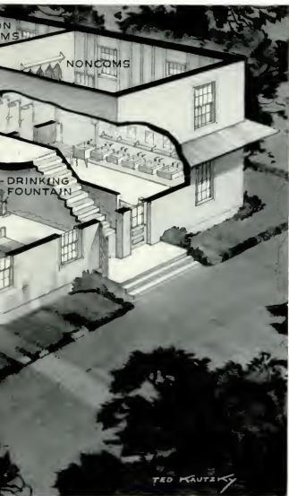
Officers and men, the Army must build 316 of these barracks. Among other buildings necessary for such a division are: 124 mess halls (170 men each), 130 storerooms, 130 day rooms, 23 officers' barracks, twelve officers' messes, 15 administration buildings, eleven Guard houses, two theaters, nine recreation buildings, one hospital (750 beds).
