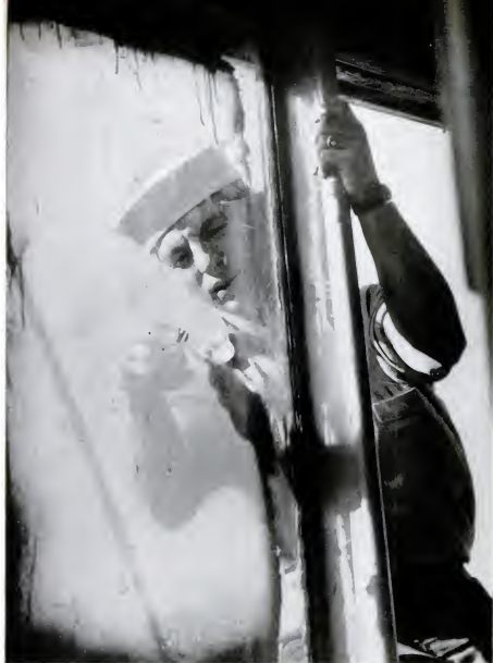
HIGH ON THE MAIN BRIDGE A SEAMAN SCRAPES PLASTIC AND ALUMINUM PRESERVATIVE OFF GLASS
