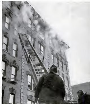
LADDER GOES UP against building on fire. The ladder extends to 85 feet and it takes two men, the driver and the tillerman, 55 seconds to crank it up.
