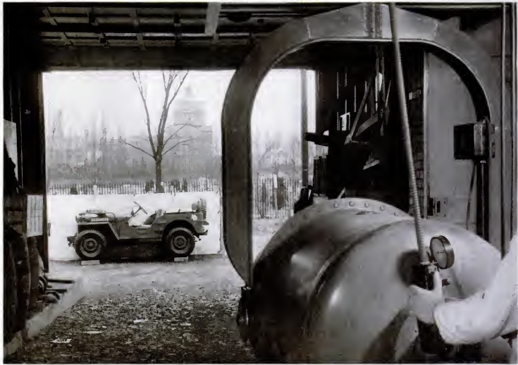
HOW THE X-RAY WAS MADE is shown in the laboratory arrangement above. In right foreground is million-volt X-ray machine aimed at jeep 60 feet away outside the lab-
