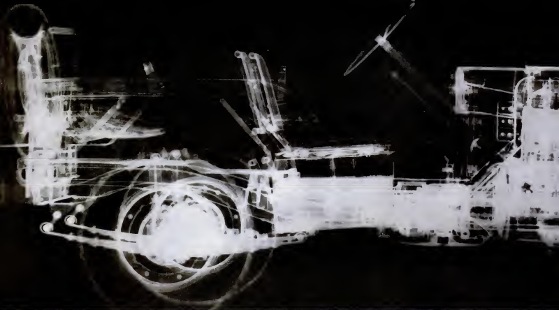
FULL-SIZED X-RAY TAKEN AT THE UNIVERSITY OF ROCHESTER X-RAY LABORATORY REVEALS THE INNER PARTS OF THE JEEP, INCLUDING ENGINE, CHASSIS FRAME AND
