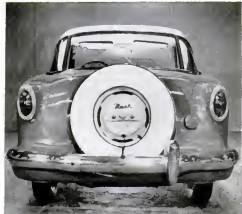
REAR VIEW of Metropolitan shows tire outside. It was in trunk in N.X.I., was moved to give more luggage space.
