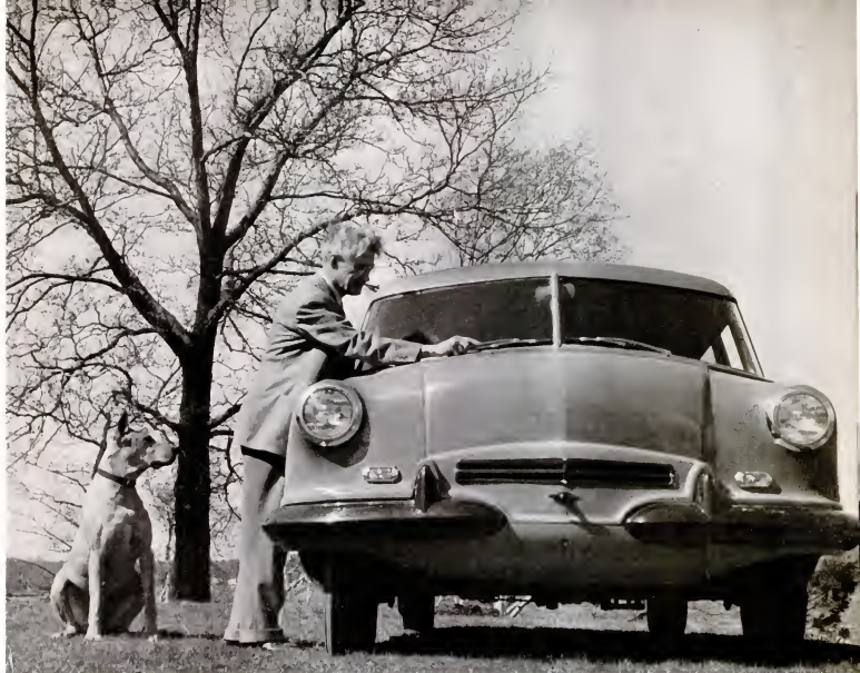
DESIGNER BILL STOUT, LIKE A SMALL BOY WITH A NEW PLAYTHING, SHOWS OFF HIS FIBER-GLASS CAR. COST OF MATERIALS USED IN BODY WAS ONLY $75
