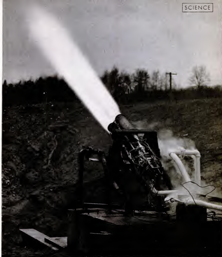
ON THE TEST STAND THE MOTOR FIRES A HARD JET OF FLAME FROM EACH OF ITS FOUR CYLINDERS. PIPE IS FROSTED BY CARRYING LIQUID OXYGEN AT -360^{\circ} F.
