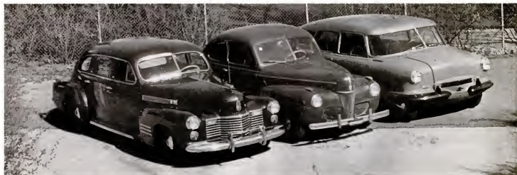
CADILLAC, FORD AND STOUT CARS (left to right) are lined up to show how Stout's rear-engine design allows for more interior space. Driver sits well forward,
