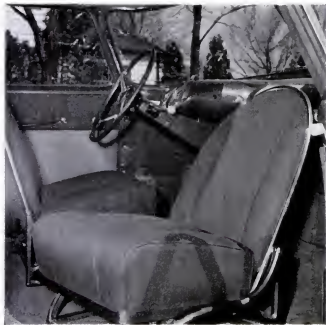
SEATING ARRANGEMENT includes movable chair which enables front-seat passenger to face to rear. Note excellent visibility through the windshield.
