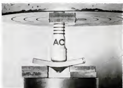
3. The thin, tapered AC insulator tip slices through the steel.
