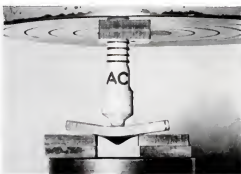
2. The heavy steel plate starts to bend as additional pressure is applied.
