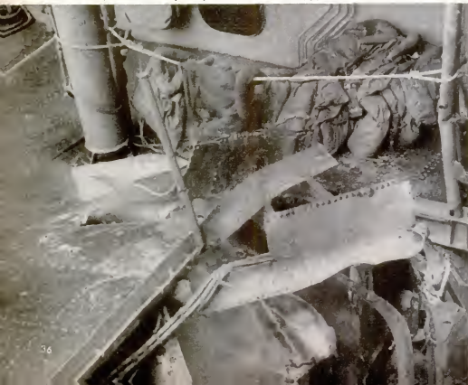
The walkway, which runs from bridge to after guns at fore-castle deck level, has been buckled upward by the force of
