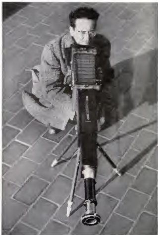
The kind of camera Feininger uses on telescopic shots must have a lens with very long focal length when large-size film is used. Lens in this 4x5 camera can be pulled out to 150 in. If he uses smaller-size film he can use a lens with shorter focal length.
