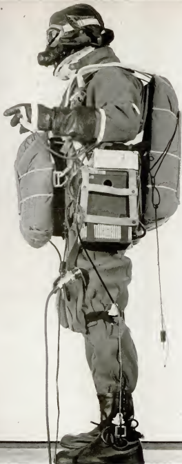
On his left hip Starnes wears a small radio transmitter wired directly to electrodes over his heart for broadcasting of heartbeats. In left hand he holds switch to cut in his voice. This arrangement broke down during fall, and only Starnes's heartbeats were clearly heard.
