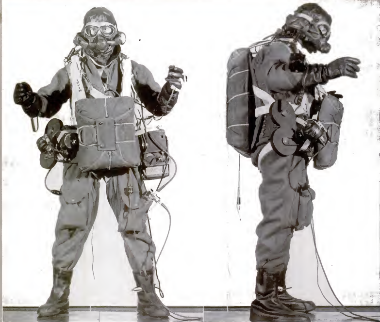
Subatmosphere Parachutist Arthur Starnes exhibits his costume before jump. His face is hidden by oxygen mask, supplied from seven-minute flask in pocket of left pant leg. Valve on flask tapped airplane's oxygen before jump. Inside his coveralls are heart and respiration recorders and barograph.
