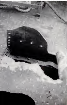
bent from normal position, is a padded chock on which whaleboat rested. The jagged chunks of metal in foreground are deck plates.
