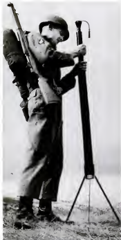
FOXHOLE DIGGER, weighing only five pounds, is erected by soldier. Fuse at top gives him 70 seconds to run.
