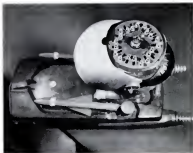
TOY'S BRAIN is a dial whose 20 push buttons can be pre-set by the operator to guide the toy along almost any desired path.
