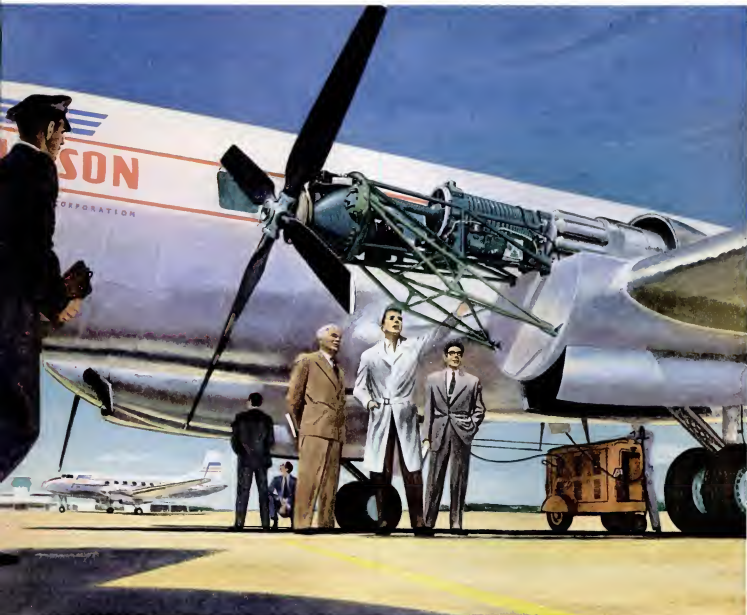
Allison "501" Turbo-Prop engines fit in nacelles of present commercial transports.
