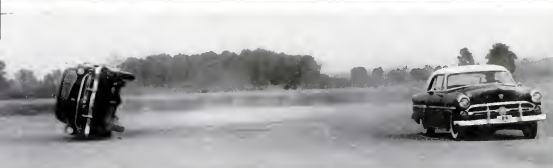
TAKING 90° CURVE AT 41 MPH, ONE CAR TIPS, AND TOPPLES. ITS TWIN, WITH CURVEMASTER, HOLDS ROAD FIRMLY
