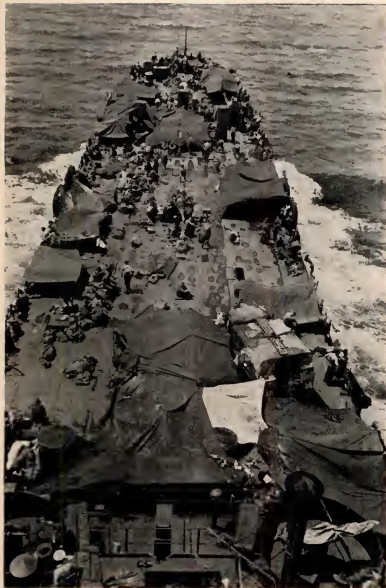
LST at 583 is packed with Australian troops resting about the deck for the fight ahead. This view, taken from above the bridge, gives a good idea of the landing ship's size and construction. Tarpaulins have been stretched along the sides to protect the men. One in center forward covers the elevator.
