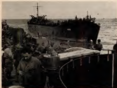
Running in at Lao , the LST opens her wide bows to be ready to disembark men and vehicles when she hits the shore. Thick vertical ramp behind the doors keeps the sea from flooding into the ship. When she is beached, the ramp will be dropped horizontally to permit the men to run across it to shore.
