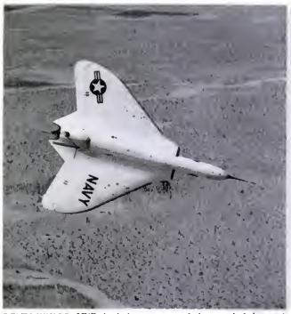
DELTA WINGS of F4D give it the appearance of a huge moth. It has an air intake on each side of fuselage, will be in full production in three months.
