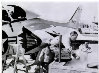
COOL FUEL , so it will contract and thus allow the jet's tanks to hold a greater load, passes through pipe which is surrounded by chunks of dry ice.
